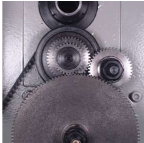
Gears set for left hand threads
