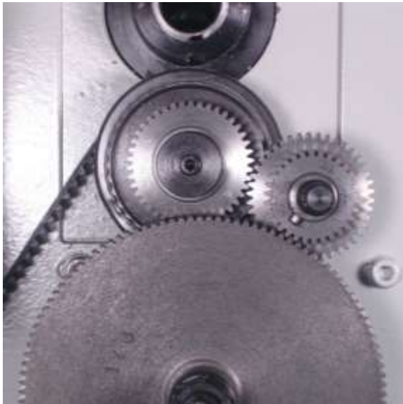
Gears set for right hand threads
